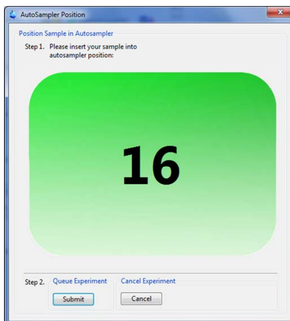
Figure 3.2: AutoSampler Position window identifies the sample position of a queued sample.
