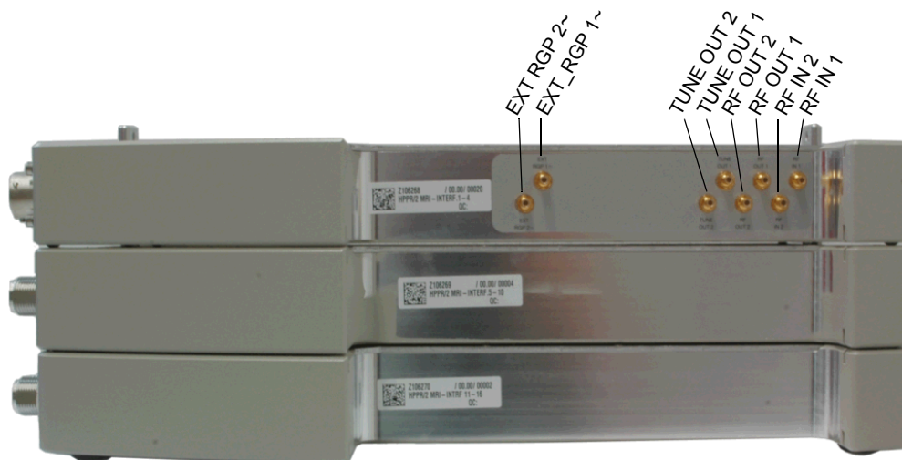
Figure 9.6. View PREAMP Connectors
