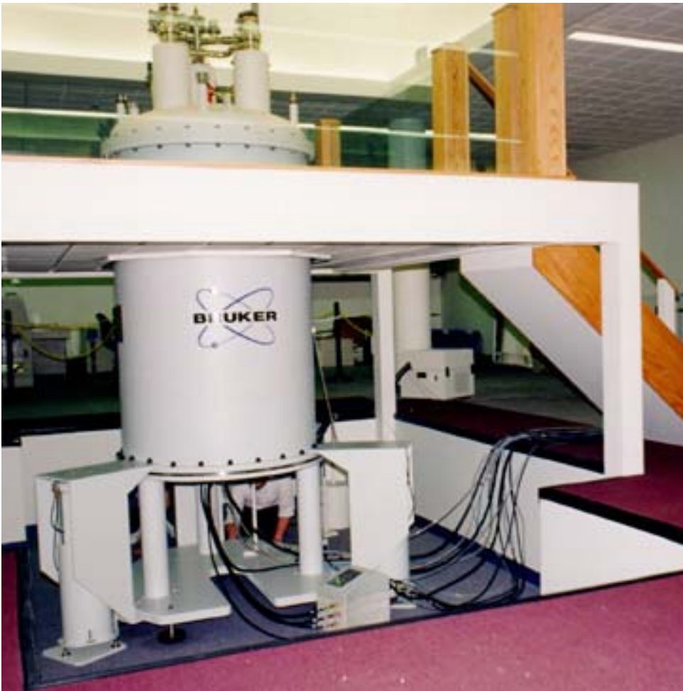
Figure 9.3: Magnet in Pit with Customized Platform
