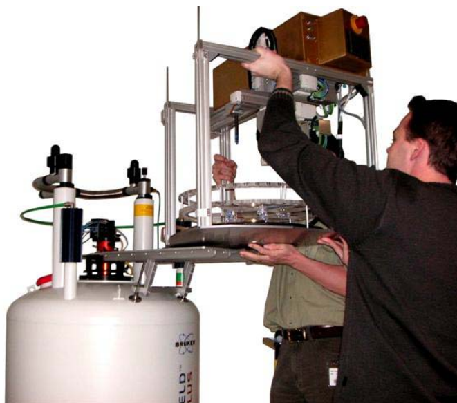
Figure 3.21. Lifting the SAMPLEJET onto the magnet
