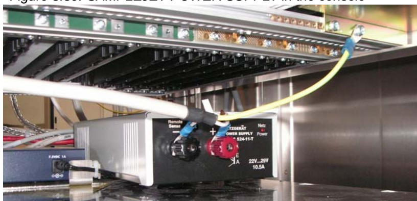
Figure 3.30. SAMPLEJET POWER SUPPLY in the console
