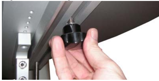
Figure 3.22. Fixing the SAMPLEJET on the platform
