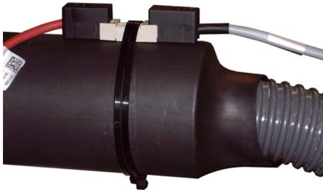
Figure 5.18. Fixing the pull-out power connector
