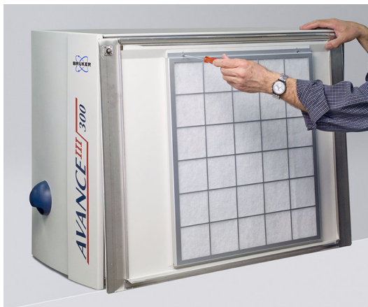
Figure 5.10. Replacement of fan filter fleece
