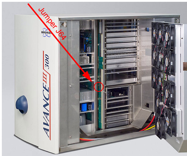
Figure 3.19. Jumper J64 installation
