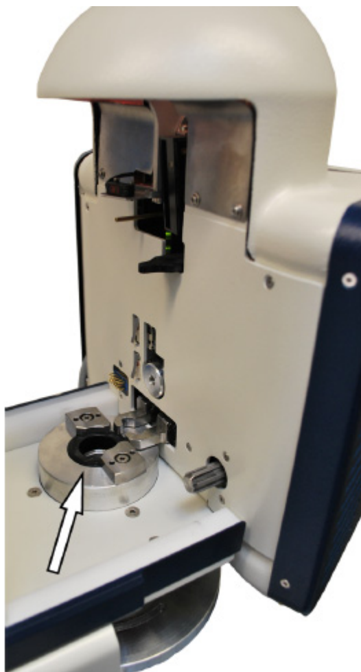
Figure 9.48 Sample Transfer Position
