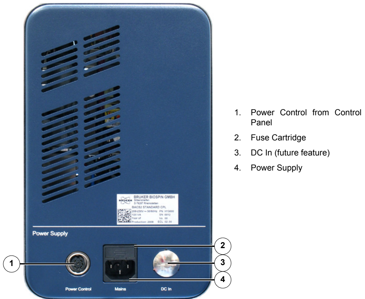
Figure 5.15 Connections Right Side
