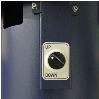
Figure 5.1: Start the Magnet Stand
