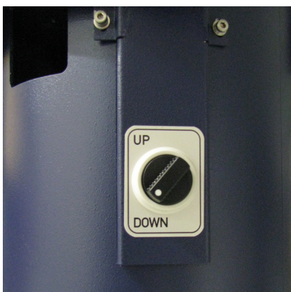
Figure 5.2: Stop the Magnet Stand
