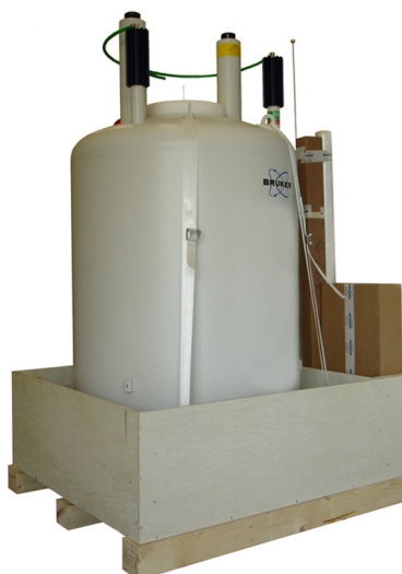
Figure 3.1: Packaging (without surrounding panels)
