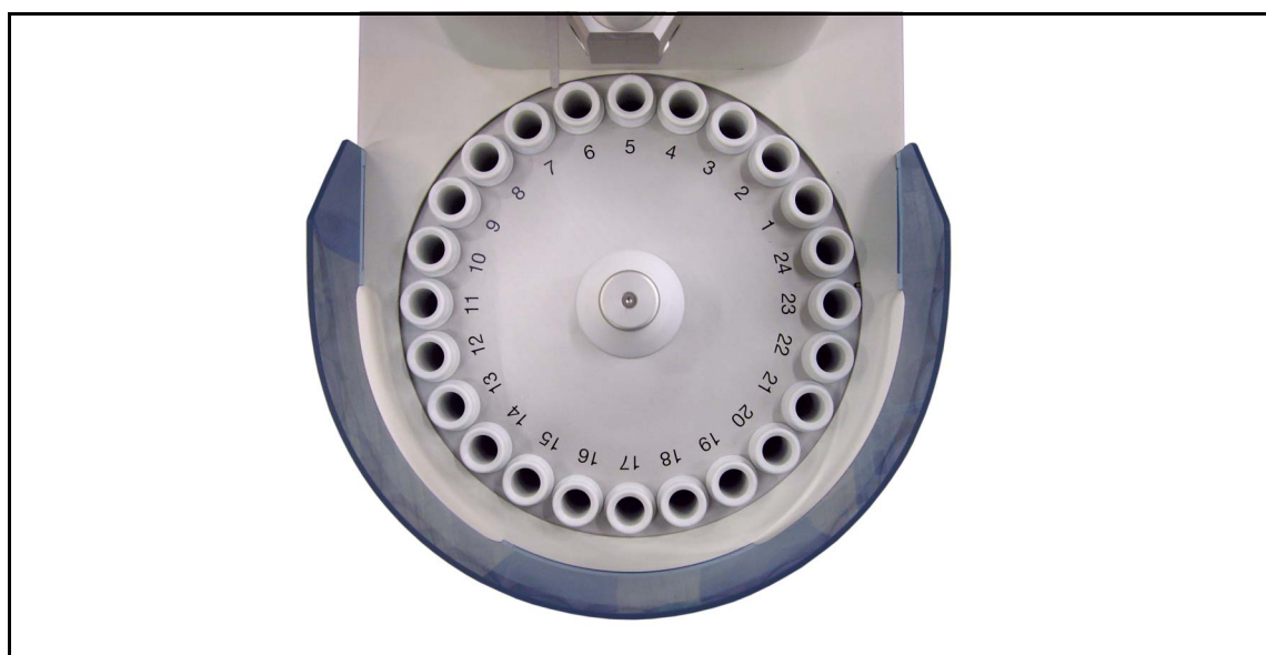
Figure 2.1: The carousel with the 24 holders
