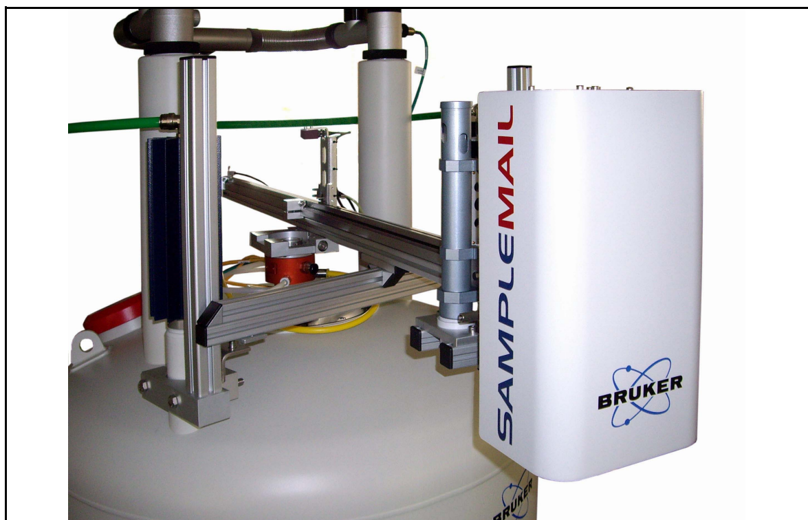
Figure 3.15: The linear axis on the magnet
