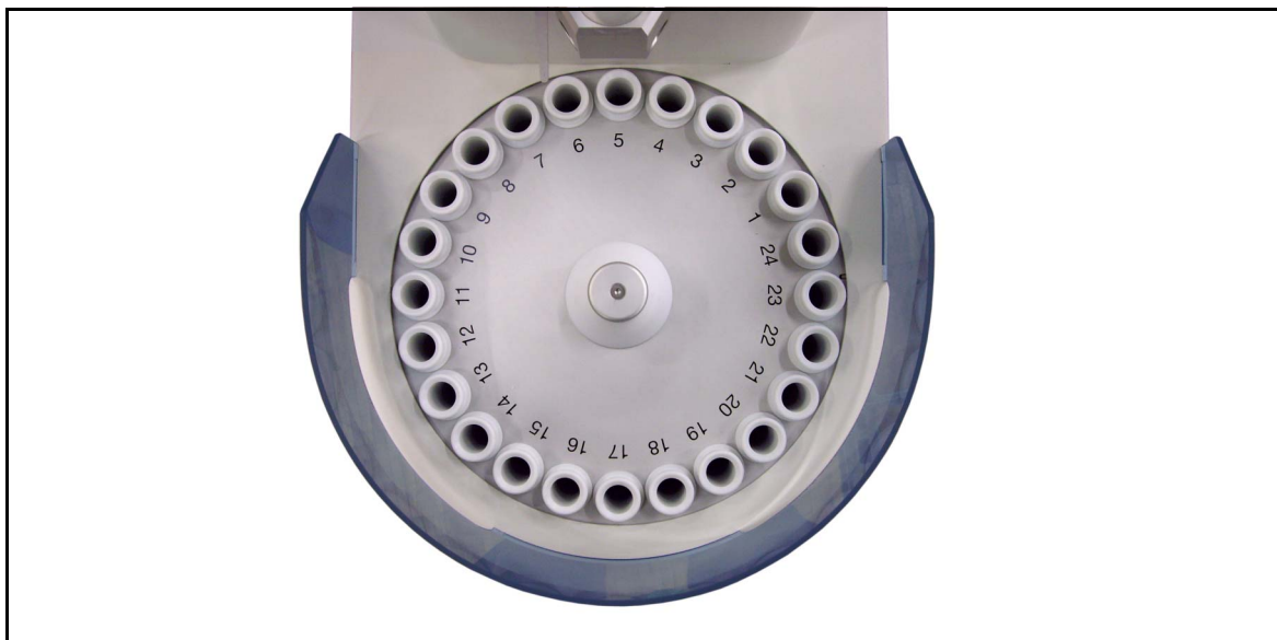
Figure 1.1: The carousel with the 24 holders
