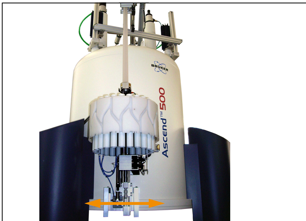
Figure 3.27: Adjust the carousel to its final position
