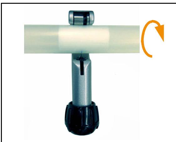
Figure 3.23: How to cut the tube with the tool
