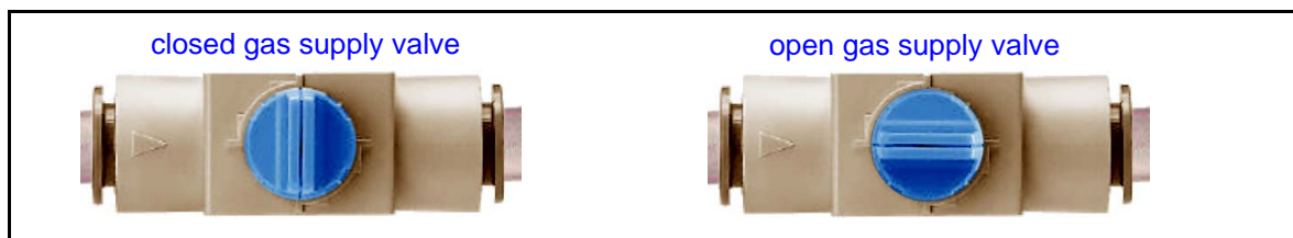
Figure 3.1: Switching on gas supply
