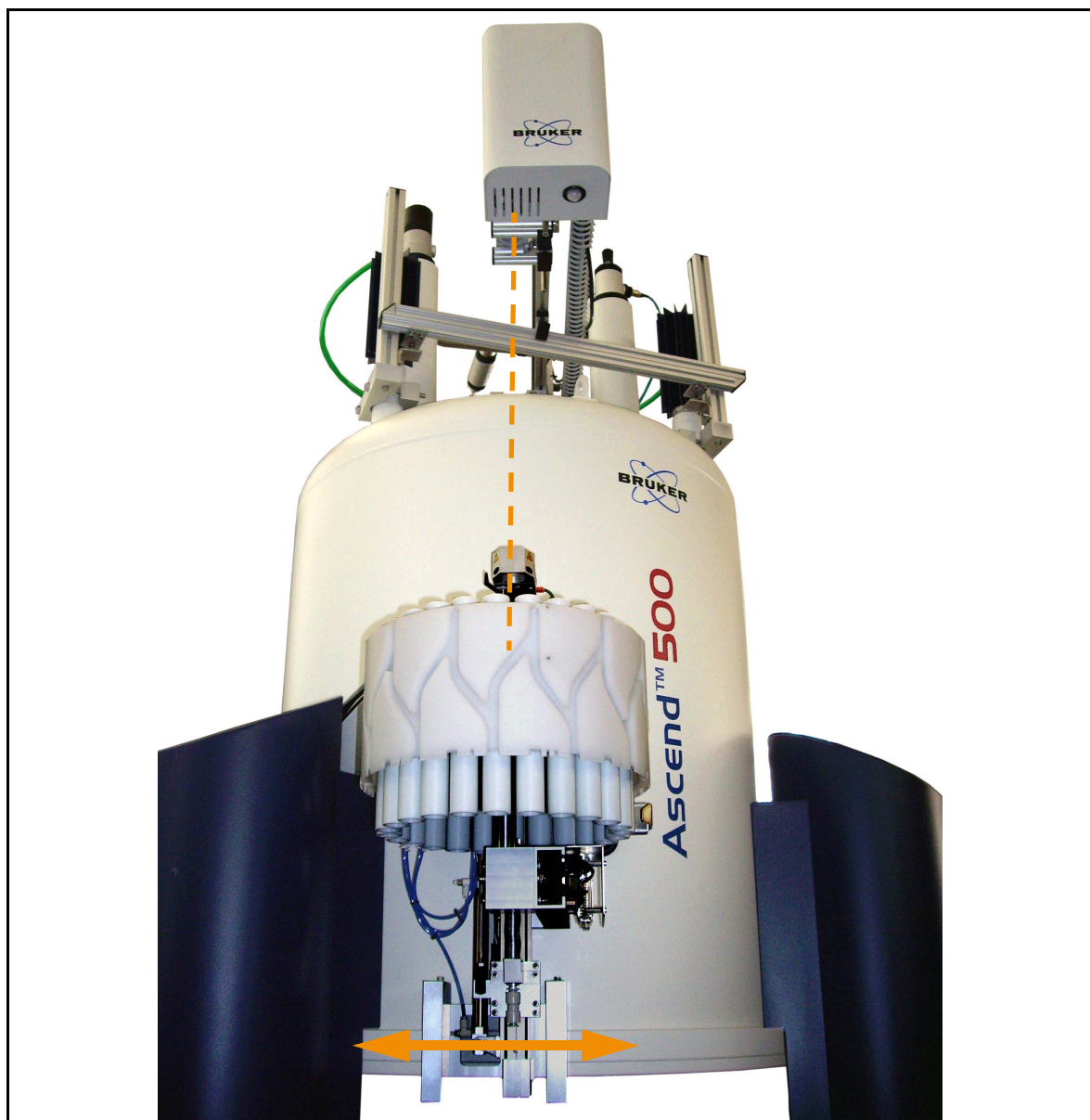
Figure 3.19: Set the carousel to its position
