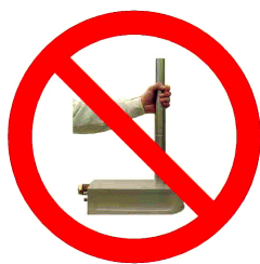
Figure 3.11. Never hold a CryoProbe at its tube!
