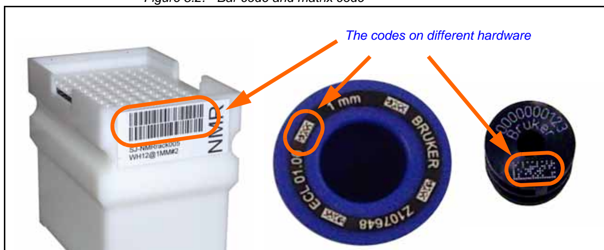
Figure 8.2. Bar code and matrix code
