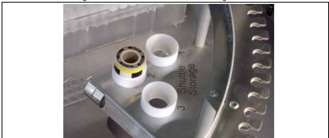
Figure 9.3. A 1mm shuttle in the Shuttle Storage
