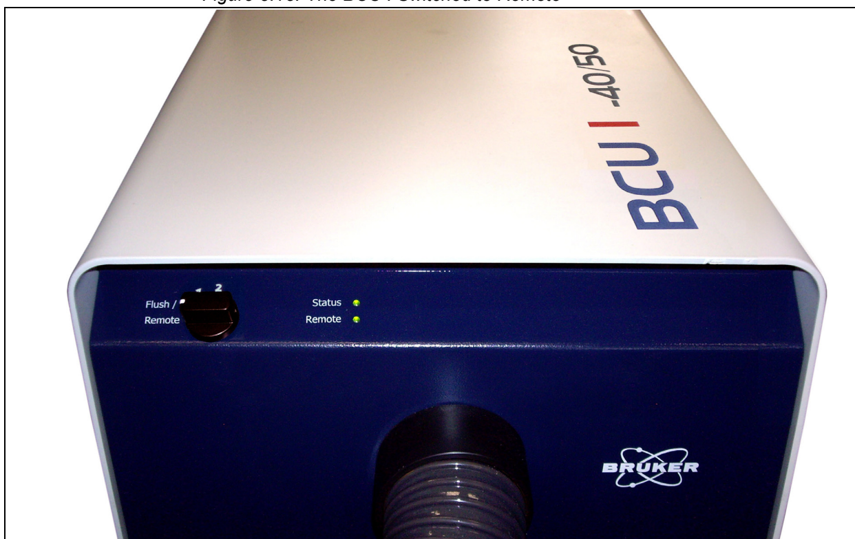
Figure 8.18. The BCU I Switched to Remote
