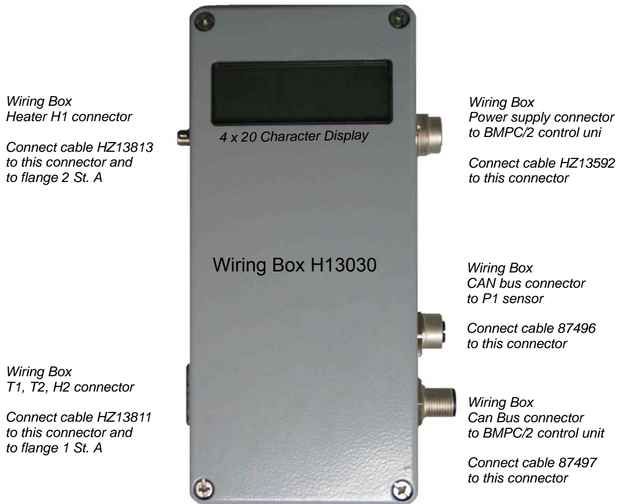
Figure 8.5 BMPC/2 Wiring Box
