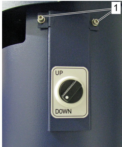
Figure 4.37: Connecting the air supply – step 6
