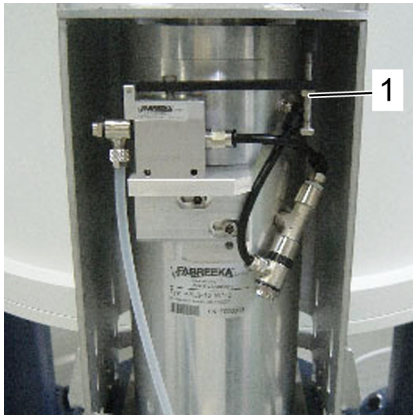
Figure 4.46: Mounting the T-safety bracket – step 6
