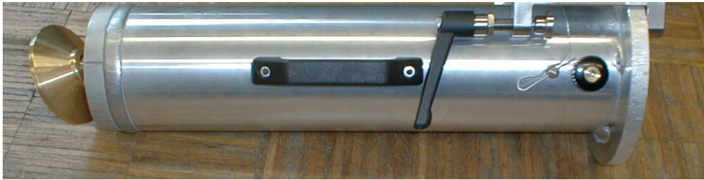
Figure 6.1: Non-ferromagnetic auxiliary repair column
