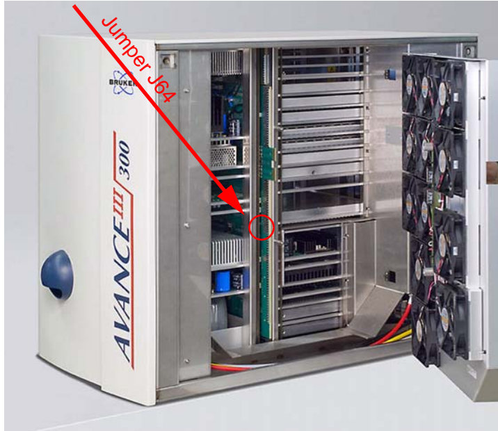
Figure 5.19 Jumper J64 installation
