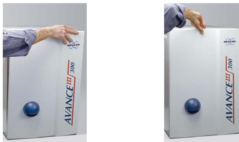
Figure 12.16 Attaching the front panel (snap in)
