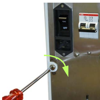
Figure 12.11 Quick snap-in fastening
