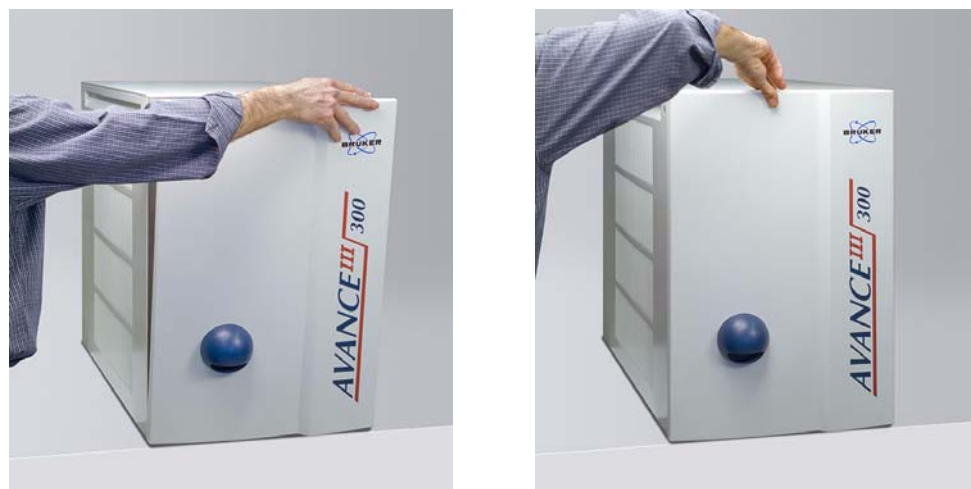
Figure 12.8 Attaching the front panel (snap in)
