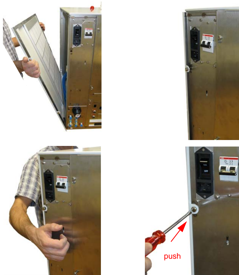
Figure 12.15 Attaching the side panels by pushing the snap in fastenings
