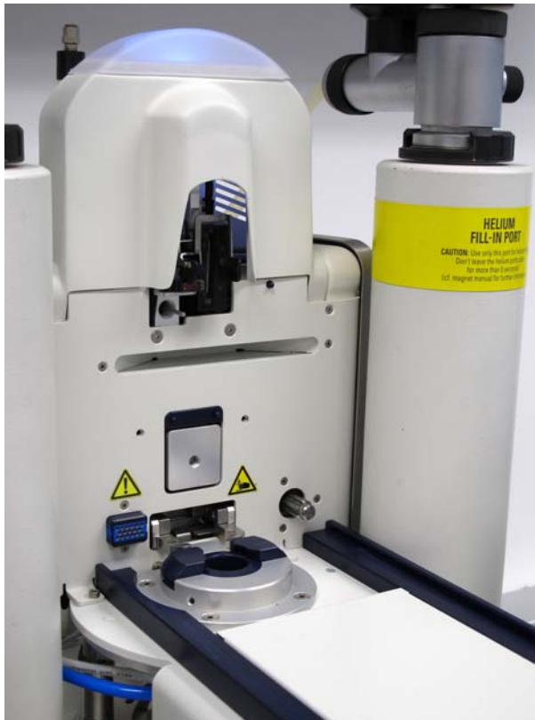
Figure 8.39: Sample Transfer Position
