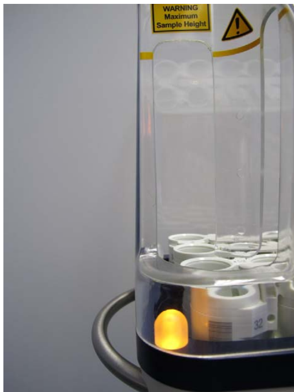
Figure 7.10: Conveyor Chain Motion Warning LED Signal
