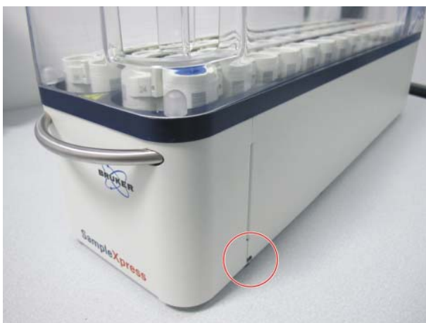
Figure 10.4: Location for Opening the Cassette Side Cover
