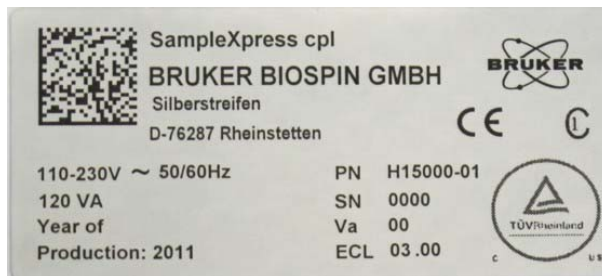
Figure 4.2: SampleXpress Rating Plate H15000-01 ECL 03.00
