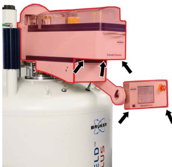
Figure 5.18: Cassette and Control Panel
