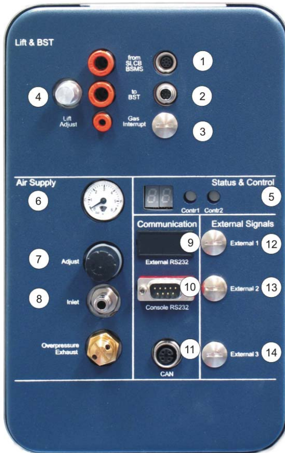
Figure 5.14: Connections Left Side
