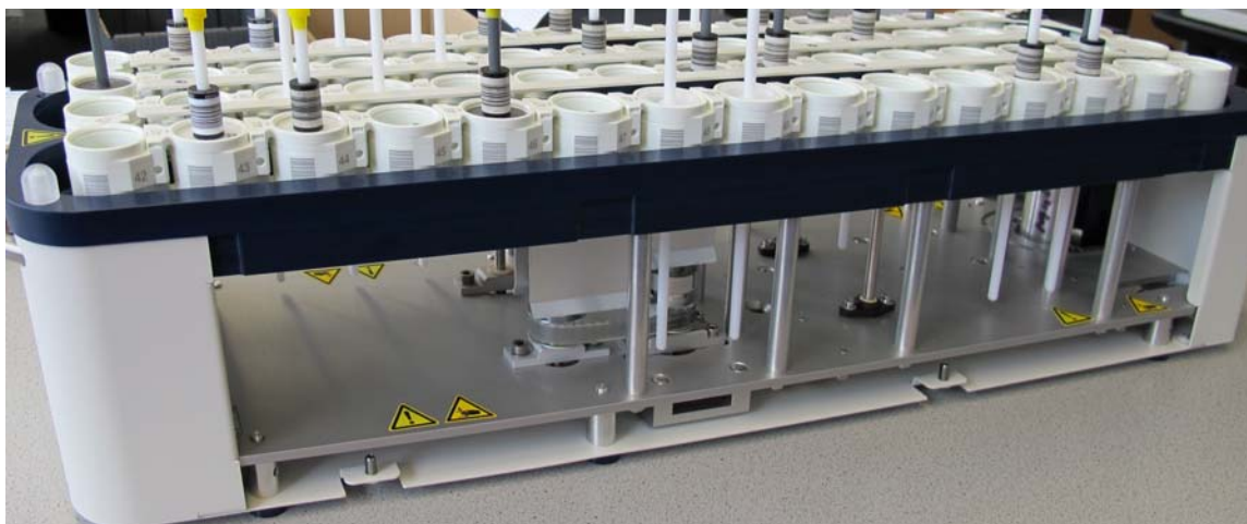
Figure 3.4: Warning Labels inside the Cassette
