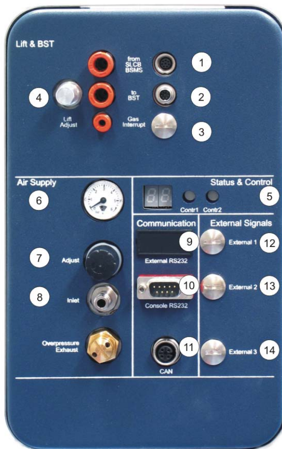
Figure 10.1: Connections Left Side
