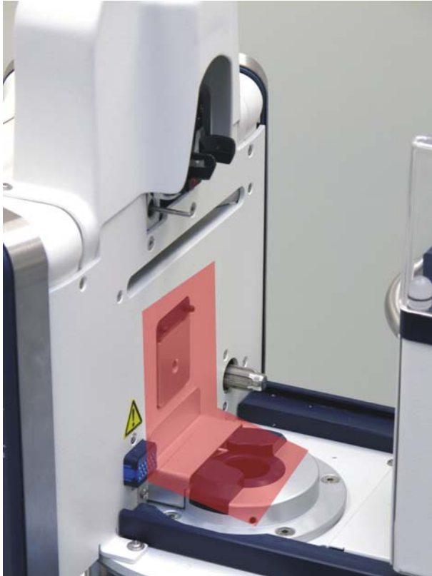
Figure 5.17: NMR Access Position
