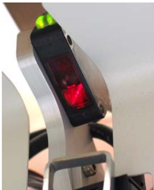
Figure 5.22 Reflex Sensor at the NMR Access Position
