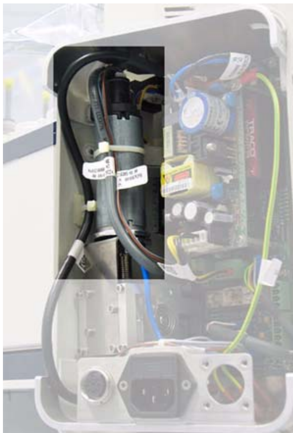
Figure 6.7 Conveyor Chain Motor
