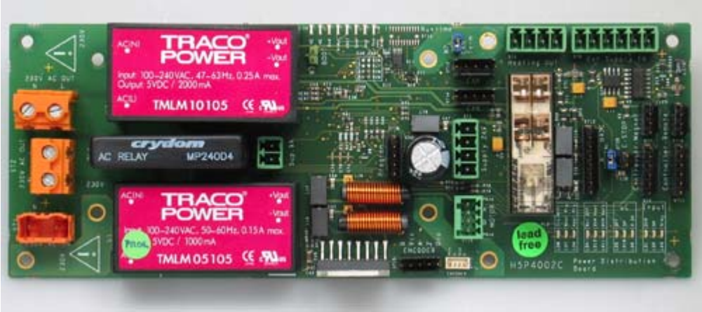
Figure 6.31 Power Distribution and Motor Control Board
