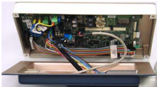
Figure 5.13 Rear of the Control Panel
