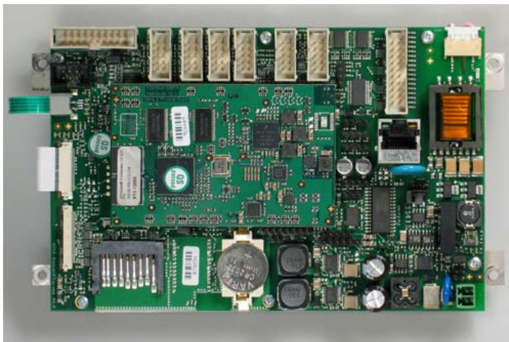
Figure 6.35 WinCE Main Controller
