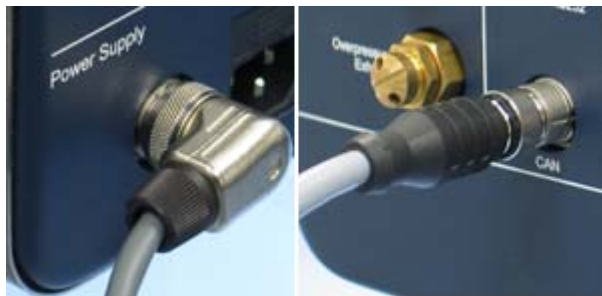
Figure 5.8 Location of the Power and CAN Cables on the Base Unit Connector Panel
