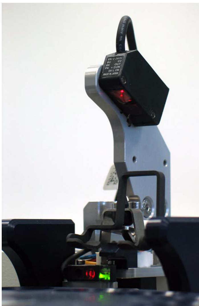
Figure 5.9 Reflex Sensor at the NMR Access Position
