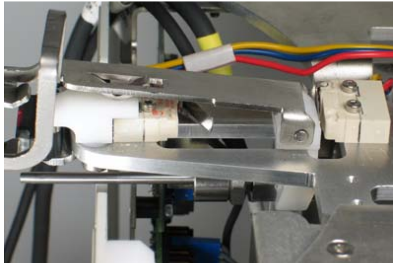
Figure 6.8 Pneumatic Cylinder End Position Microswitches
