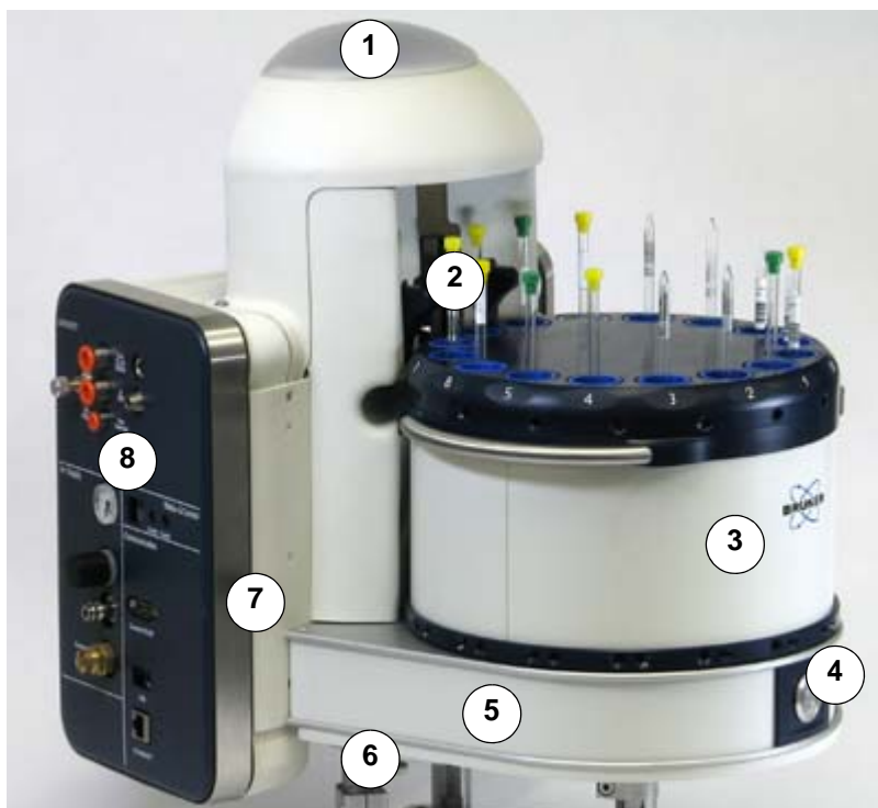
Figure 6.1 SampleXpress Lite Main Components
