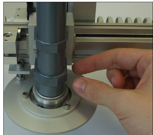
Figure 1.29: Correct Adjustment: The CALIBRATION RING has dropped down
