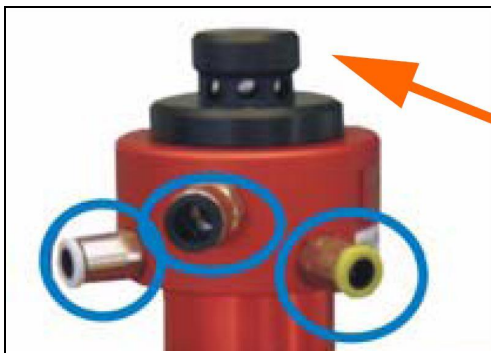
Figure 1.5: Magnet secured with the protection lid.
