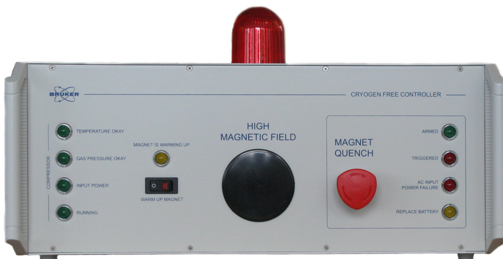
Figure 5.8: Bruker Cryogen Free Controller (BCFC) – Front View
