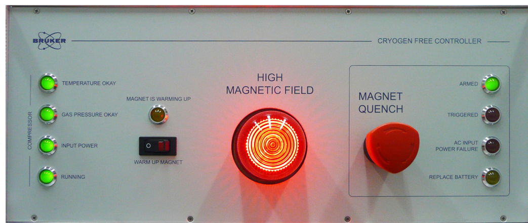
Figure 5.16: Energizing the magnet and checking the indicator
