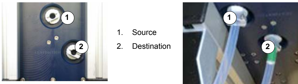
Figure 6.16 Exchange Unit - Source and destination
