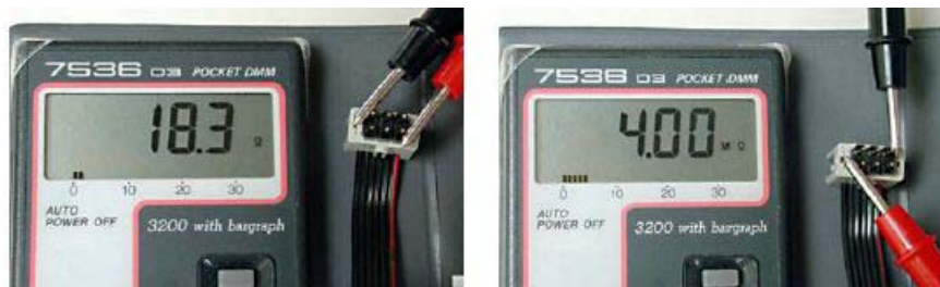
Figure 10.28 Measuring the Inner Coil (left) and Encoder Resistance (right)
