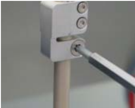
Figure 9.48 Fasten the Clamp Part on the PEEK Adapter
