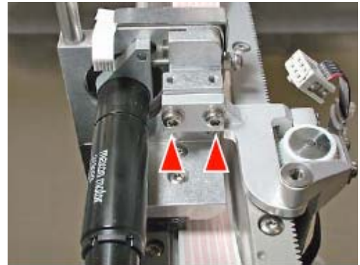
Figure 9.34 Y-motor support with mounting screws
