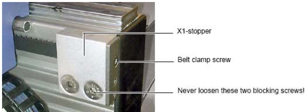
Figure 9.13 Loosening the Belt Clamp
