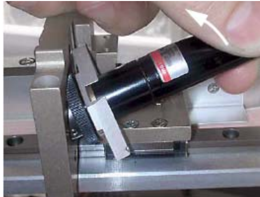
Figure 9.40 Removing the Z-Motor Assembly
