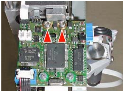
Figure 9.33 YZ-board connectors and screws
