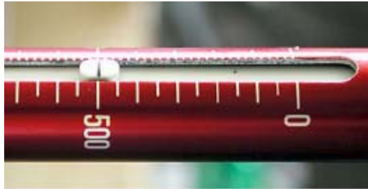
Figure 10.8 Spring-Loaded Scale Indicator
