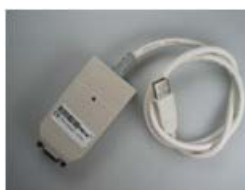
1 x P/N: O10375 - USB CAN interface controls the robot.
