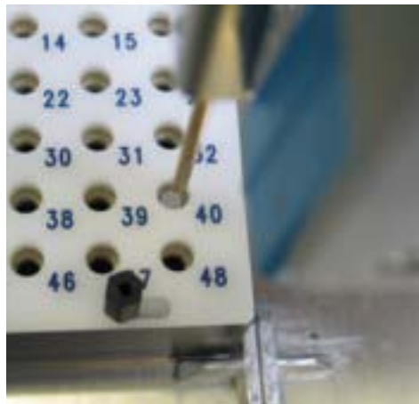
Figure 8.2 Checking the XY position over the rotor position
