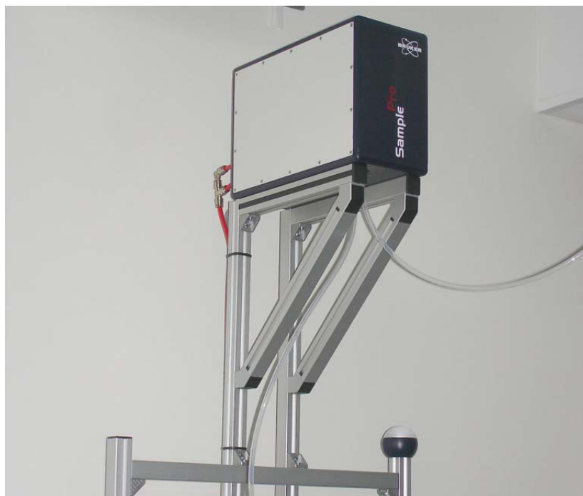
Figure 6.12 Exchange Unit After Mounting
