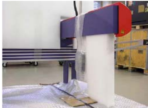
Figure 15.7 Strapping down the device and supporting the arm with a foam block.
