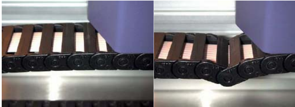
Figure 9.22 Caterpillar Drive Chain Perfectly Shaped Figure 9.23 Buckled Caterpillar Drive Chain
