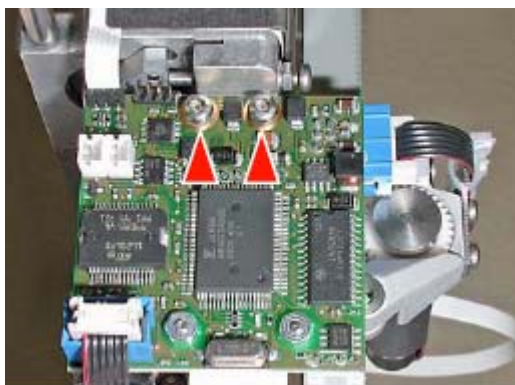
Figure 9.30 YZ-board connectors and screws
