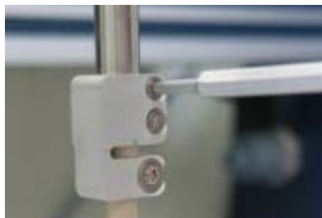
Figure 9.46 Disassembly of the Pickup Adapter
