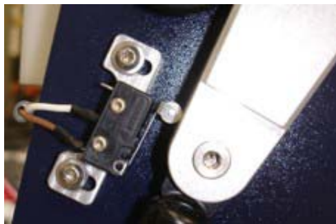
Figure 9.54 Door Open Sensor
