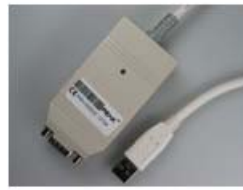
1 x P/N: O10375 - USB CAN interface controls the exchange unit.
