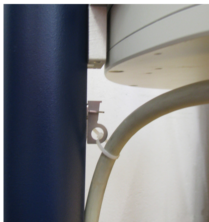
Figure 4.27: Fix the cable to the clamp in the opening slit of the pillar
