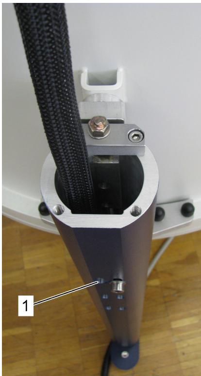
Figure 4.24: Guide the cable through the pillar
