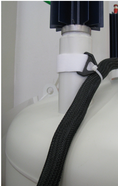
Figure 4.23: Arranging the cable routing at one of the N 2 turrets
