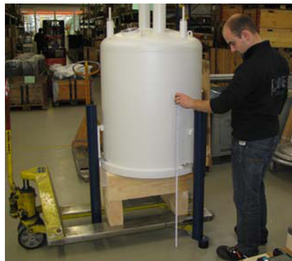
Figure 4.17: Check the height of the cryostat
