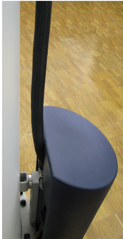
Figure 4.29: Cable routing after mounting the pillar covers
