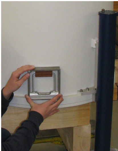
Figure 4.20: Leveling the cryostat
