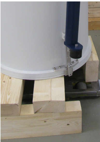
Figure 4.11: Mounting the pillars to the cryostat
