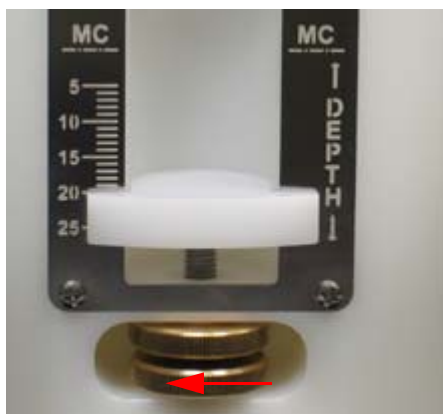
Figure 7.4 Loosening the Knurled Screws
