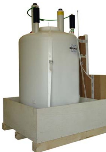
Figure 3.1: Packaging (without surrounding panels)
