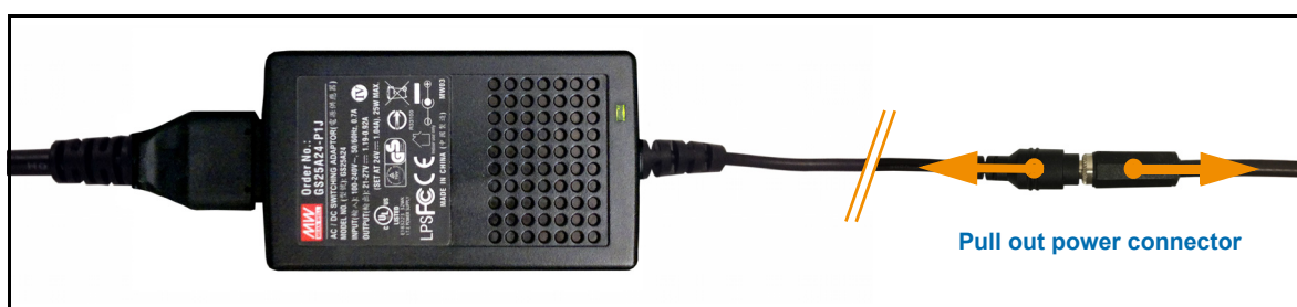
Figure 3.9: Interrupting the Power Supply
