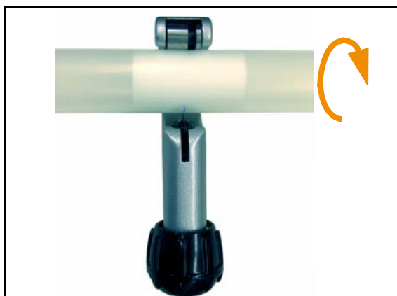
Figure 3.8: How to Cut the Tube with the Tool
