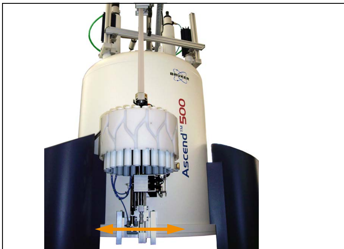
Figure 4.23: Adjust the Carousel to its Final Position
