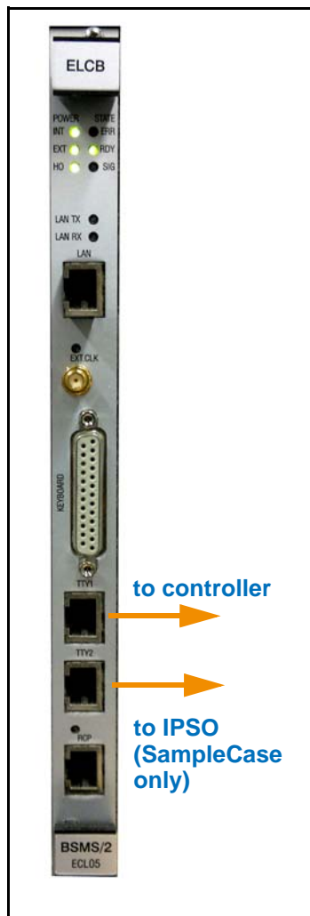
Figure 4.27: Connections on the ELCB
