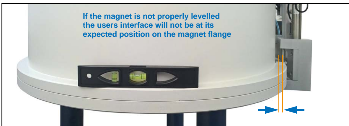
Figure 3.4: Consequences of Unlevelled Magnet II
