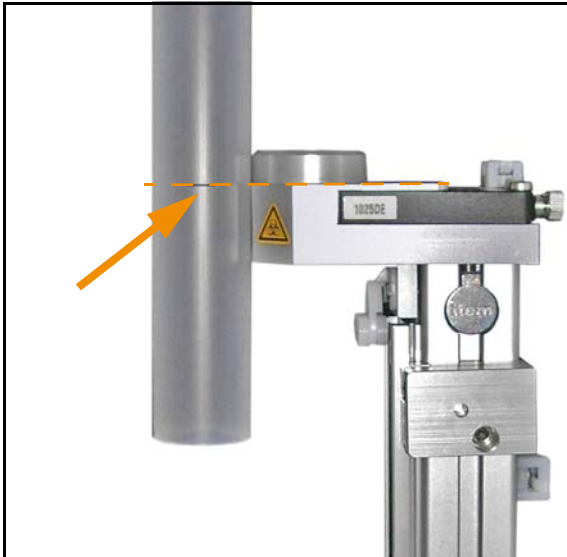
Figure 4.12: Mark the Tube for Cutting
