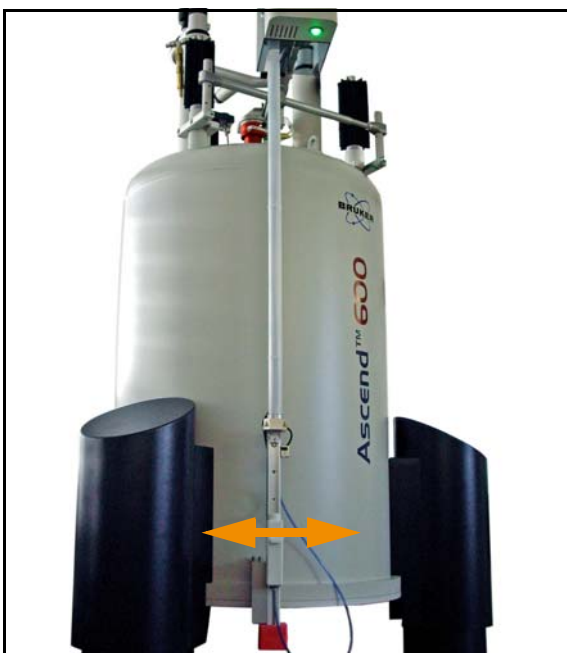
Figure 4.13: Adjust the Hand Slider to its Final Position
