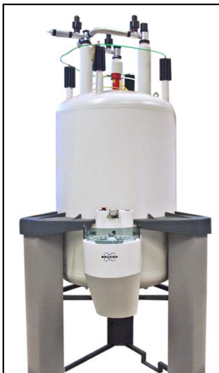
Figure 5.4: SampleCase on a Round Bottom Magnet.
