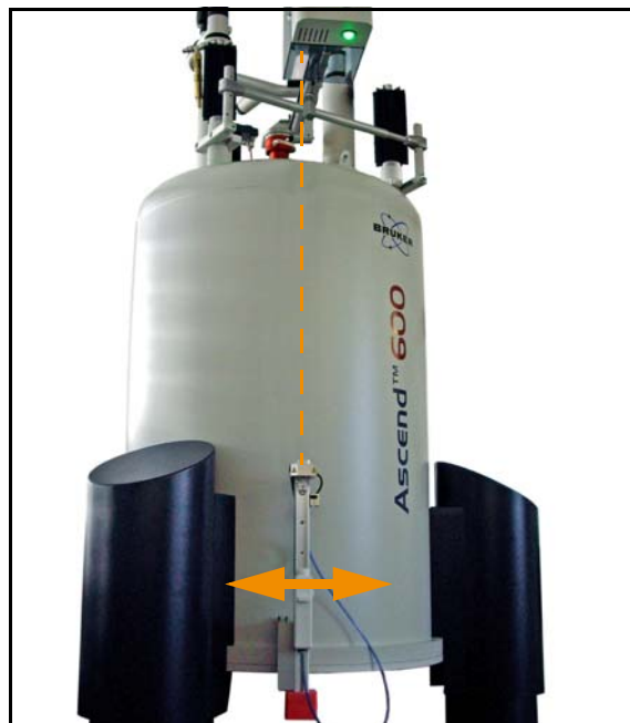
Figure 4.11: Set the Hand Slider to its Position
