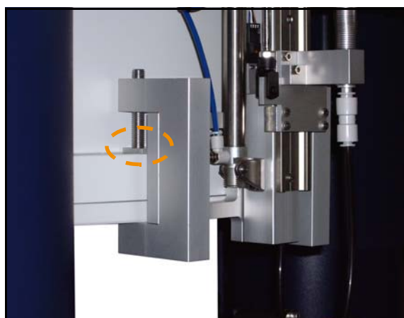
Figure 4.16: Clamping the Carousel on the Magnet
