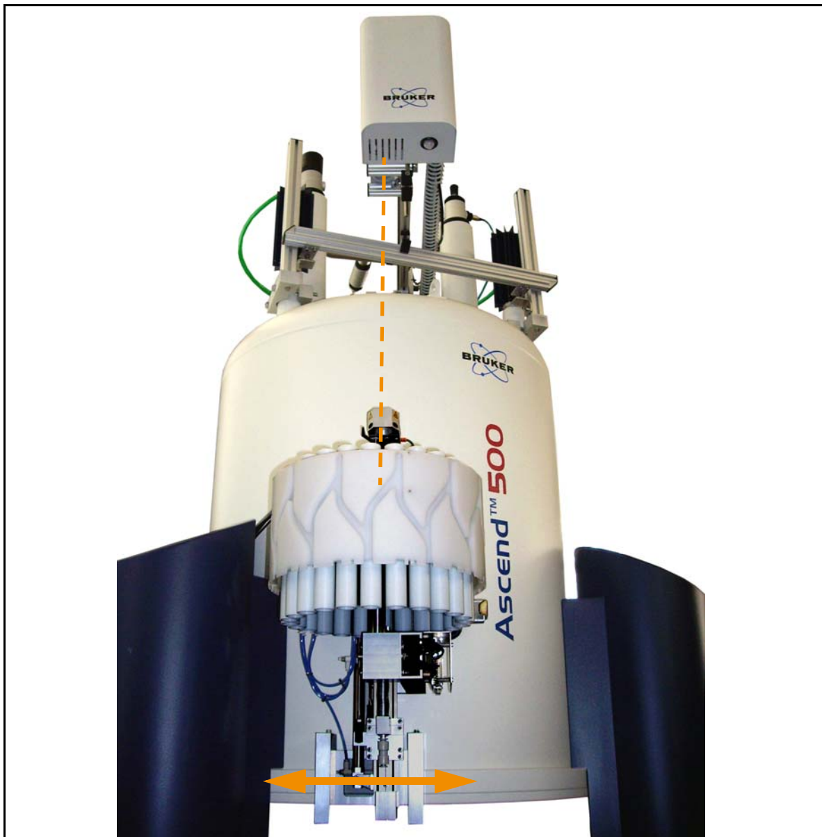
Figure 4.17: Set the Carousel to its Position
