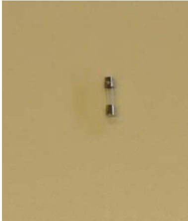
Figure 10.2: Fuse 5x20 mm 4.0AT P/N 2257 2:
