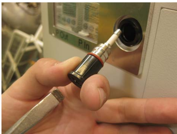
Figure 9.4: Cryocooler Controller Fuse
