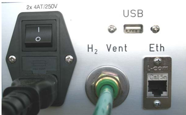
Figure 6.2: H 2 Gas Vent Outlet
