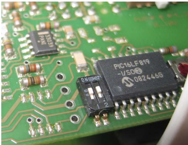
Figure 5.4: Configuration Switches on the Printed Circuit Board
