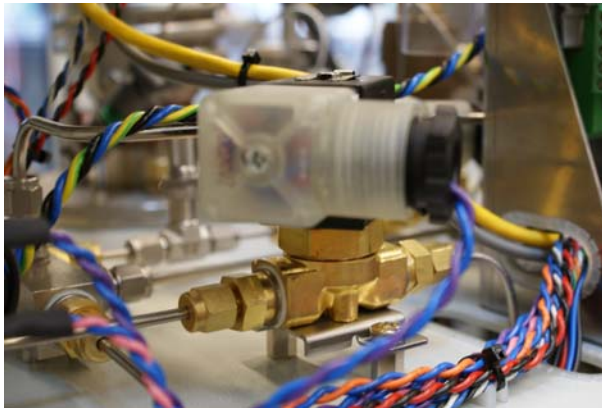
Figure 7.5: Gas Valve with Electrical Connector
