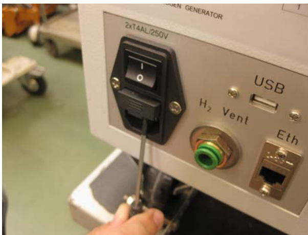
Figure 8.5: Opening the Line Fuses Holder
