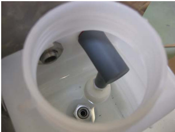
Figure 4.3: Coolant Fluid Level Switch
