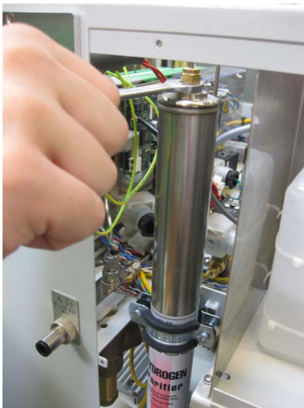
Figure 7.6: Gas Purifier Cartridge
