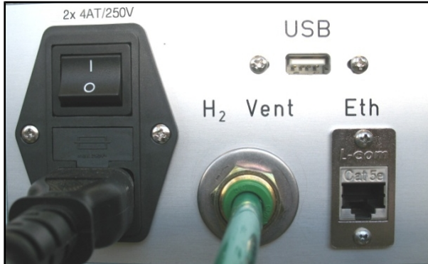
Figure 6.2: H2 Gas Vent Outlet
