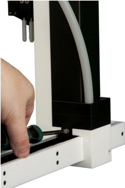
Figure 9.3: Attaching the Z-Drive to the Carriage.
