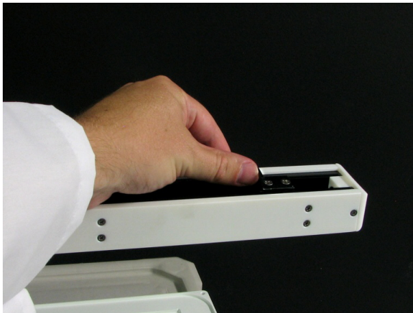
Figure 9.1: Positioning the Carriage.
