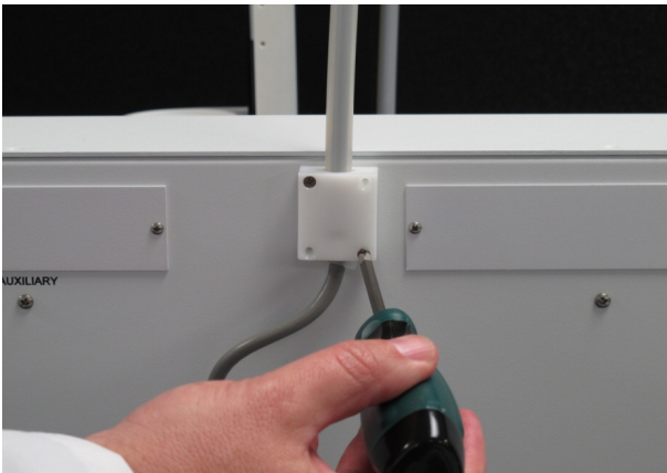
Figure 9.4: Attaching the Z-Drive Strain Relief Block
