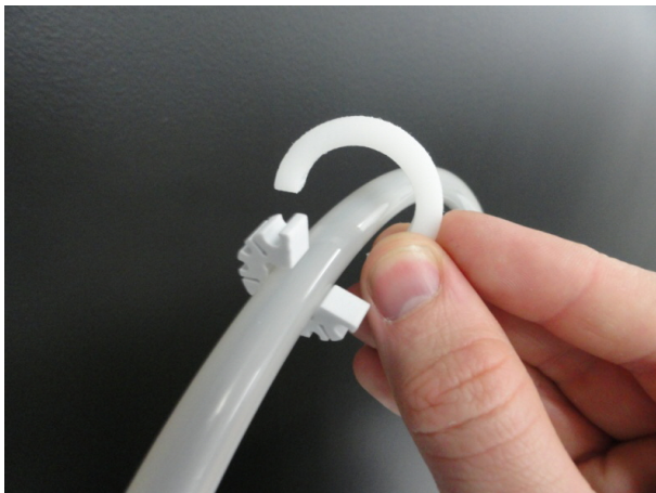
Figure 9.6: Connecting Tubing Tamer
