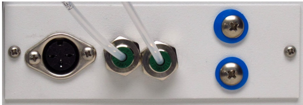
Figure 9.8: Gripper Tubing Connection on Back of Autosampler
