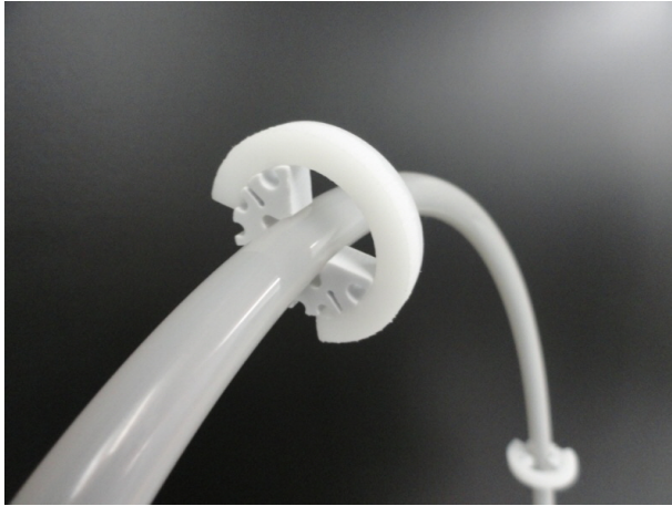
Figure 9.7: Tubing Tamer Properly Installed on Z-Drive Cable
