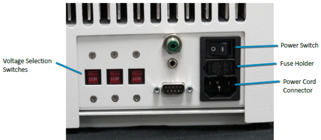
Figure 6.5: Power Connections for the Unit
