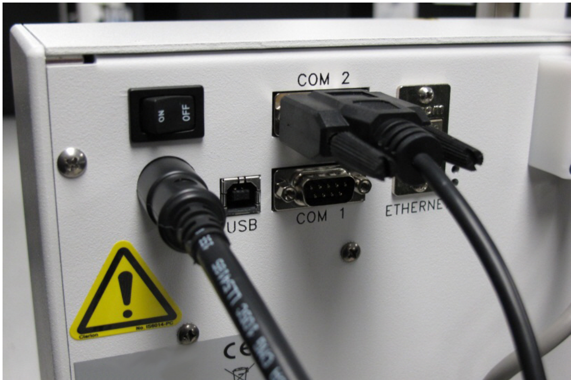
Figure 6.3: Serial Cable Connected to the Back of the Autosampler.
