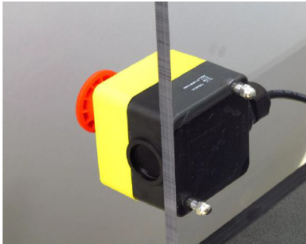
Figure 7.5: Rear View of E-Stop After Mounting (Shown mounted to safety barrier so that screw locations are more visible)
