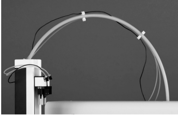
Figure 9.11: Tubing After Installation
