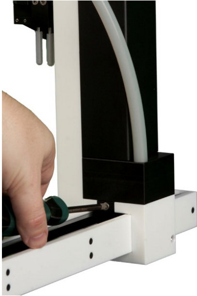
Figure 9.3: Attaching the Z-Drive to the Carriage.
