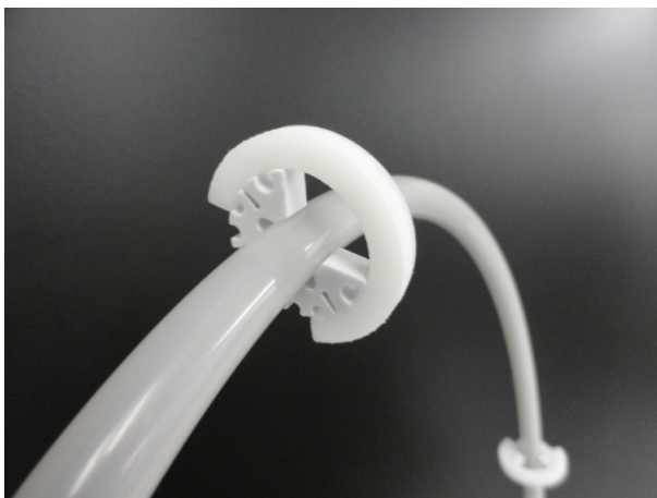
Figure 9.7: Tubing Tamer Properly Installed on Z-Drive Cable
