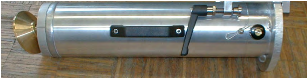
Figure 6.1: Non-ferromagnetic auxiliary repair column
