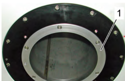
Figure 8.2: Disassembling the RT Tube - step 1
