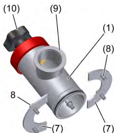
Figure 4.25: Mounting the Vacuum Valve
