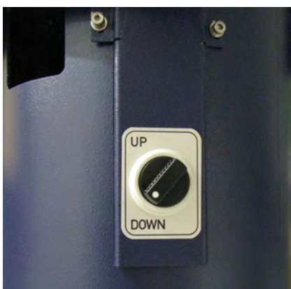
Figure 5.3: Stop the Magnet Stand
