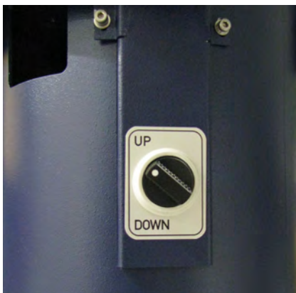
Figure 5.2: Start the Magnet Stand
