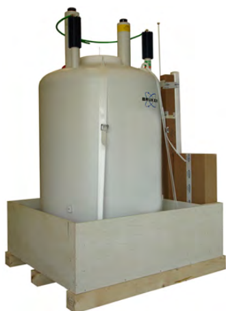
Figure 4.2: Preparing the Cryostat
