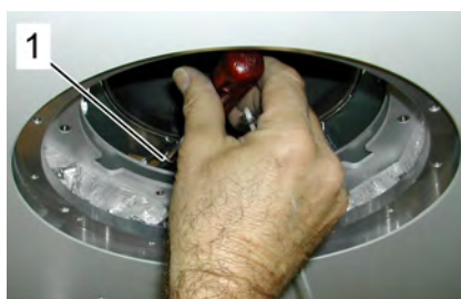
Figure 4.14: Assembling the Nitrogen Tube - step 5
