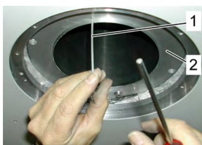
Figure 4.13: Assembling the Nitrogen Tube - step 4
