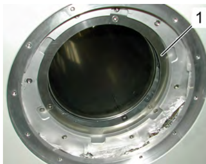
Figure 8.6: Disassembling the Nitrogen Tube - step 3
