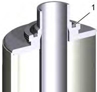
Figure 4.30: Mounting the Helium Level Sensor - step 1
