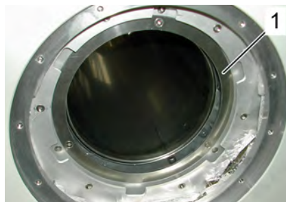
Figure 4.10: Assembling the Nitrogen Tube - step 1
