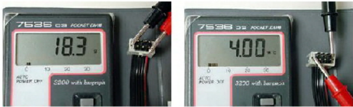
Figure 11.25: Measuring the Inner Coil (left) and Encoder Resistance (right)
