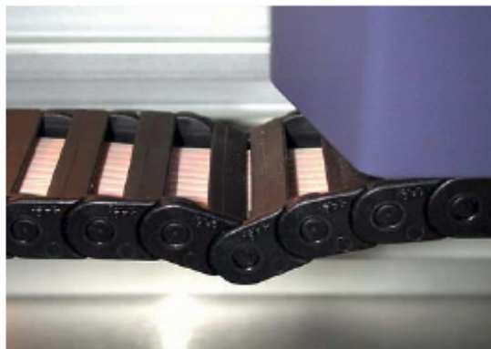
Buckled Caterpillar Drive Chain
