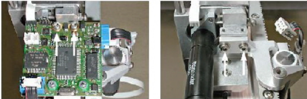
Figure 11.19: YZ-Board Connectors and Screws (left) and Y-Motor Support with Mounting Screws (right)
