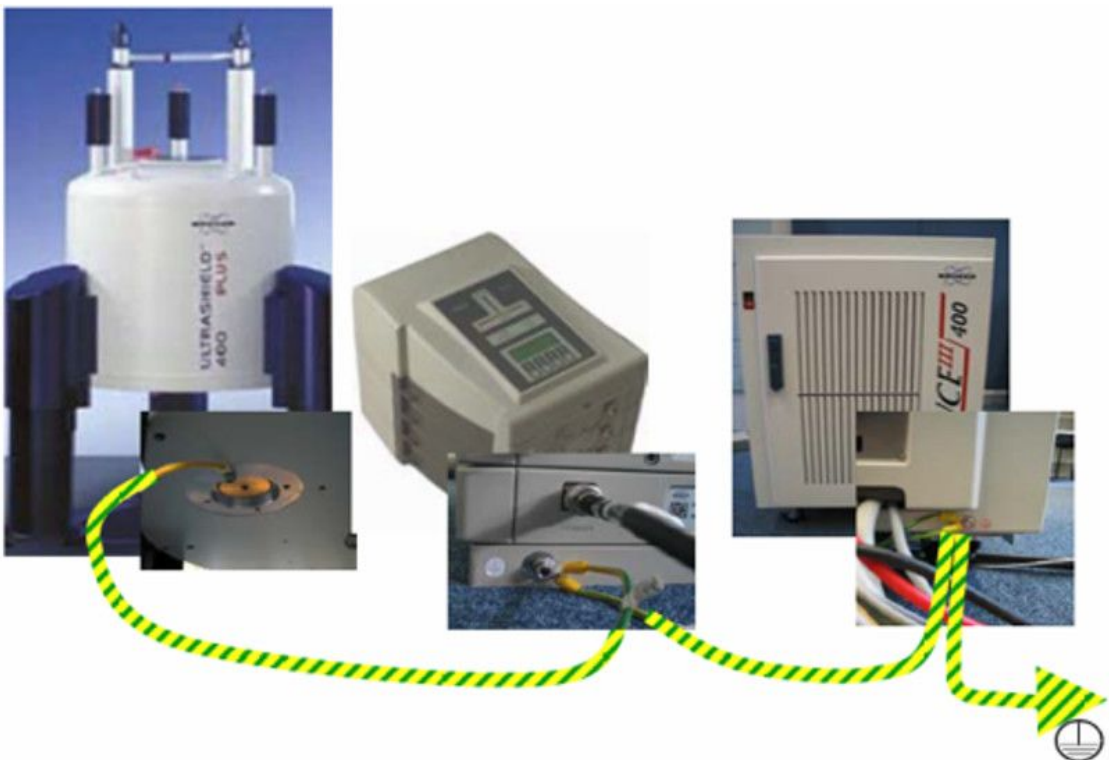
Figure 3.2: AVANCE Spectrometer with External Preamp (HPPR/2)
