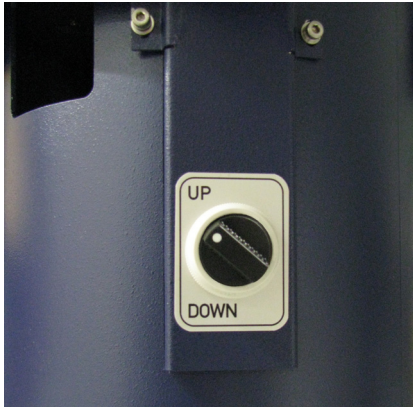
Figure 5.1: Start the magnet stand
