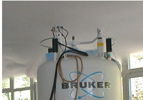
Figure 6.1: Magnet system during a quench
