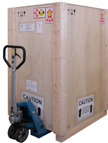
Figure 3.2: Transportation by Forklift - front side
