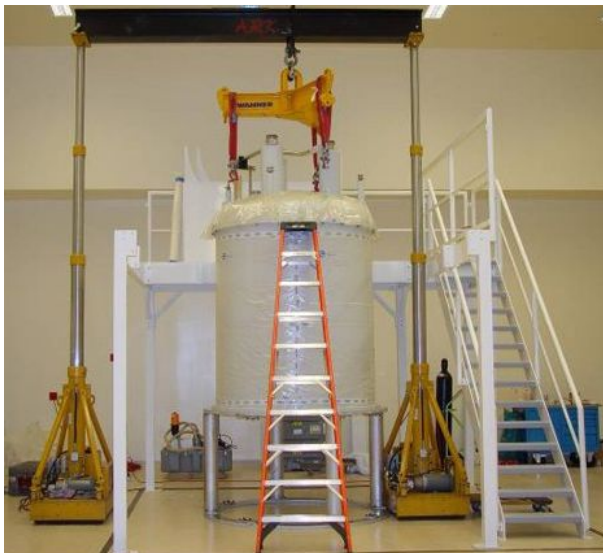
Figure 5.1: Area of Maximum Ceiling Height Needs to be Extended to Allow for the Lift System's I-beam
