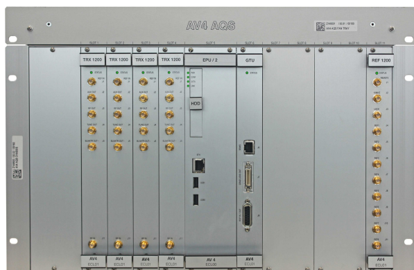
Figure 4.1: Typical AV4 AQS Chassis configuration for 4-Channel AV NEO.
