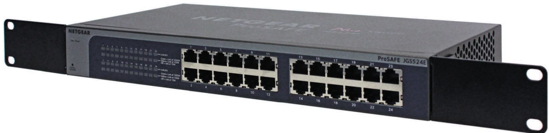
Figure 14.1: View ETHERNET SWITCH 24-Port
