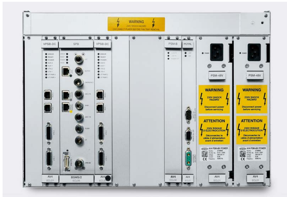
Figure 4.2: AV4 BSMS Chassis Rear View
