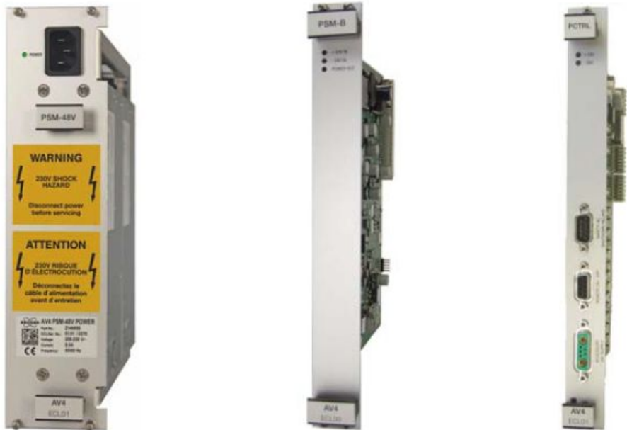
Figure 7.1: BSMS Power Supply Modules Overview
