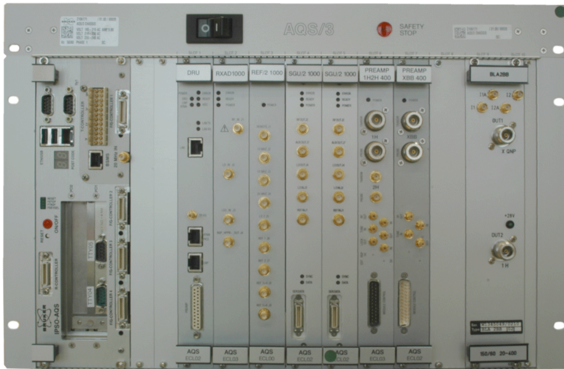
Figure 2.2. 2 Channel AQS/3 with RXAD and DRU
