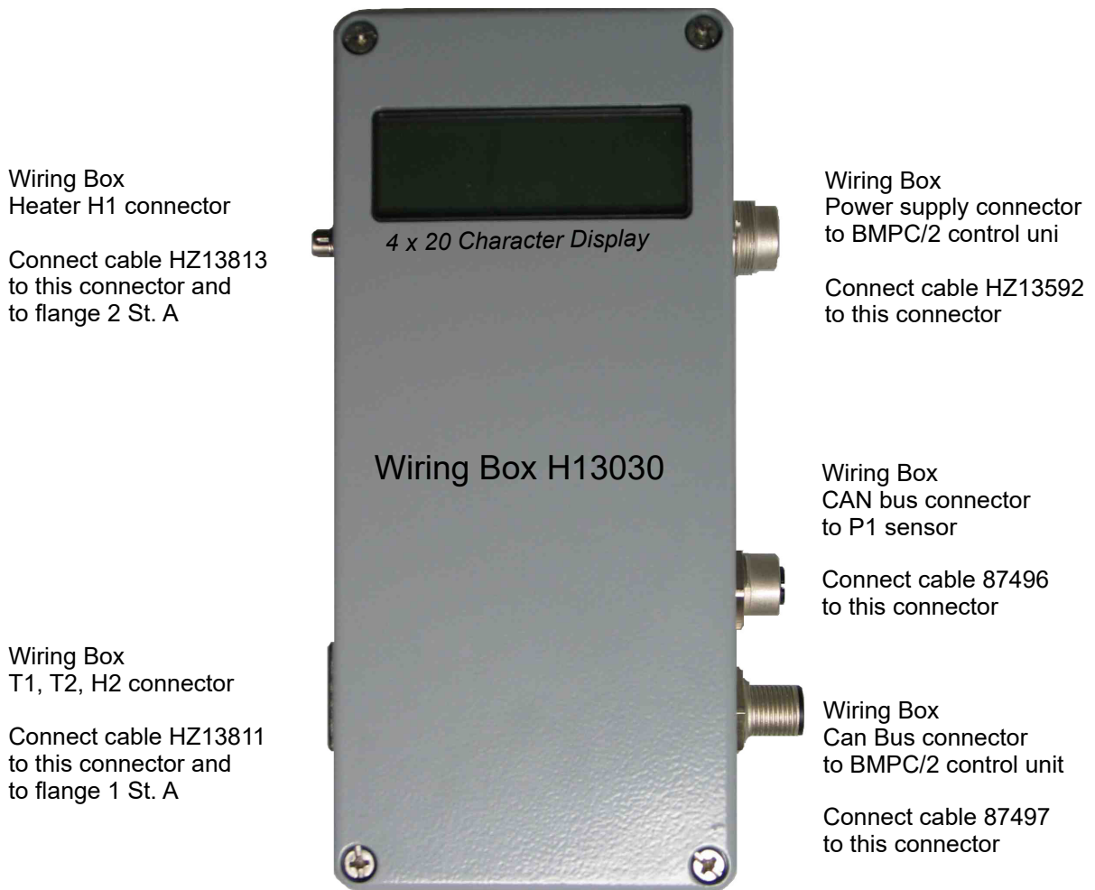
Figure 5.6: BMPC/2 Wiring Box
