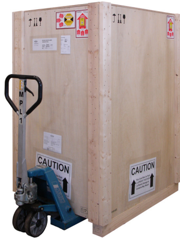
Figure 3.2: Transportation by fork lift – front view
