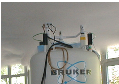
Figure 6.1: Magnet system during a quench
