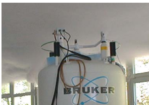
Figure 6.1: Magnet system during a quench
