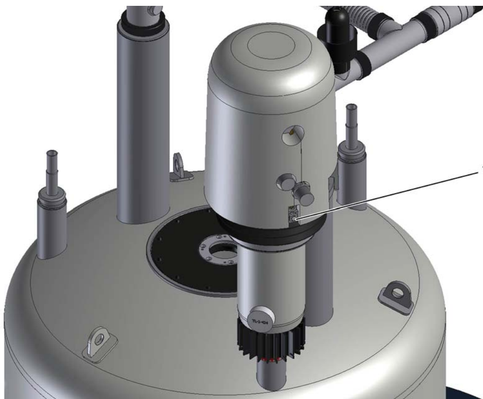
Figure 2.1: BNL safety device
