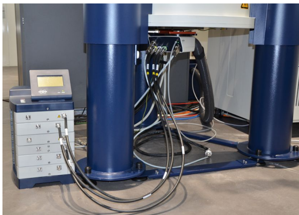
Figure 6.1: iProbe installed in the magnet
