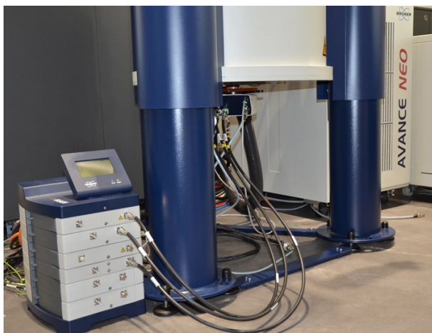
Figure 5.3: iProbe installed in the magnet
